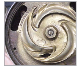
Competitor Impeller is effectively worn out.
