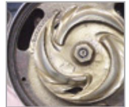
Competitor Impeller is effectively worn out.
