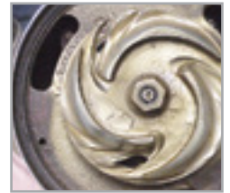
Competitor Impeller is effectively worn out.
