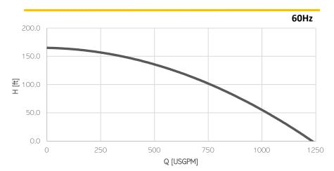
Model EL354 Brake Power [kW|HP] 37 | 49 Electric Power [kW|HP 40 | 53 Frequency [Hz] 60 44% Efficiency [%] Number of Poles 4 RPM 1758 Voltage [V] 575 Rated Current [A] 48,0 Solid handling [mm|in] 35 | 1.4 Discharge [DN-PN] 100-10
