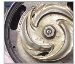
Competitor Impeller is effectively worn out.
